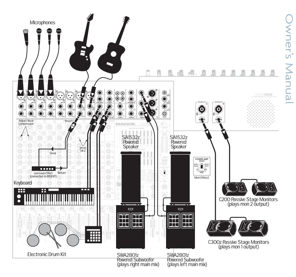
This diagram shows microphones attached to the mic inputs of channels 1 to 4, electric guitars connected directly to ch. 7 and 8 (with hi-z switch pressed in), a line-level effect connected to ch.7 insert, a keyboard attached to channels 9/10, and an electronic drum kit attached to channels 11/12. Add vocal compression as required, by tweaking the compression knobs on channels 1 to 4.
